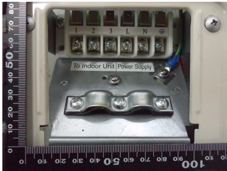
28. RAV-GM301ATP-E, RAV-GM301ATJP-E, RAV-GM301ATP-TR, Main supply terminal and Terminal block for interconnecting cable and cord anchorage
